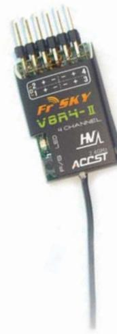
**Note:** Voltage out equals to voltage in. Be sure that when using battery or regulated output from ESC, the capacity must meet the usage conditions of servos.
