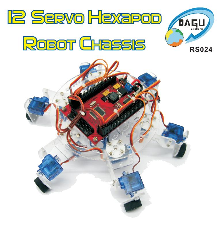
The 12 DOF Hexapod robot chassis from DAGU is a simple, low cost robot chassis designed for students and novices. Simple sample code for Arduino compatible controllers allows the chassis to be driven in any direction using common TV remotes.
