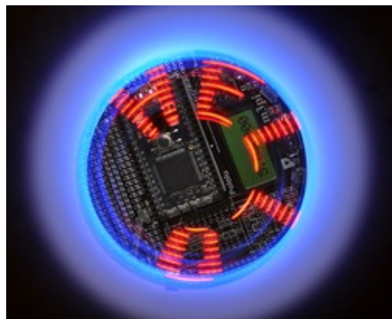
Pololu m3pi robot writing "HELLO" with its eight mbed-controlled LEDs as it spins in place (persistence of vision).
