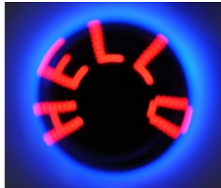
Pololu m3pi robot writing "HELLO" with its eight mbed-controlled LEDs as it spins in place (persistence of vision).
