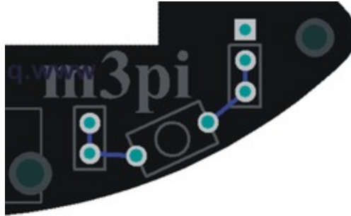
General-purpose pushbutton on the m3pi expansion PCB.
