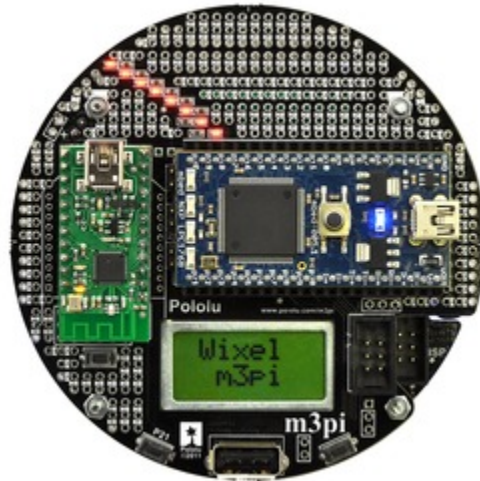
Pololu m3pi robot with mbed and Wixel modules socketed.
