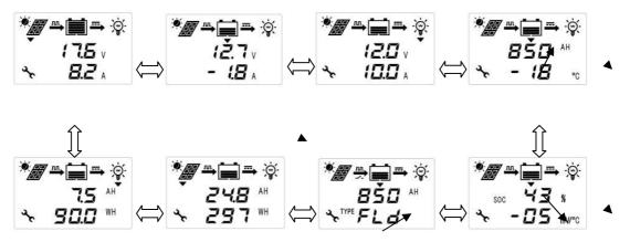
The data can be adjusted: battery capacity AH, battery temp. compensation, battery type. On read status, press K1/SET for setting data.
