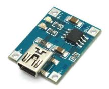
The module is used for charging of single lithium battery or multiple lithium batteries in parallel, and the charging port can take power from the USB port.
