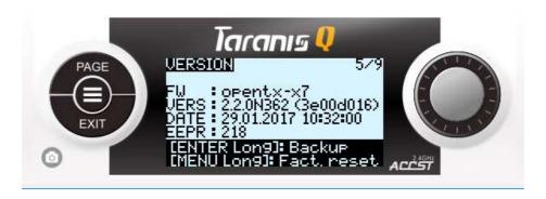
here you can check the FW version you currently have on the radio. "VERS" should correspond to the version you've just uploaded.
