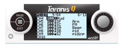
Interpretation: CH9 of the receiver would receive 100% (full range) of S2 pot input (from -100 (negative endpoint) signal at S2 full to the left to +100 (positive endpoint) signal at S2 full to thw right. With 0 (center) signal at center detent point).
