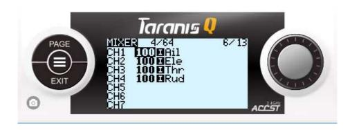
This screen is a core of all model channel behavior. Whenever we want to make any changes to the way the channel outputs are functioning – we would have to create or edit our mix for the corresponding channel. Now, if you have followed this document – you see the same mixes as shown on the screenshot. Only 4 mixes for 4  $1^{\rm st}$  channels in AETR order. This shows us that first 4 channels are already working... Let me explain how it interprets. Let's take the first line:
