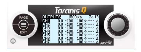
I would take CH1 (Aileron) as an example: highlight this channel, press "ENTER" to go into the edit.
