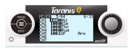
Interpretation: CH5 of the receiver would receive 100% (full range) of SF switch input (-100 (negative endpoint) signal at SF switch at down (far from you) position and +100 (positive endpoint) signal at SF switch at up (close to you) position).
