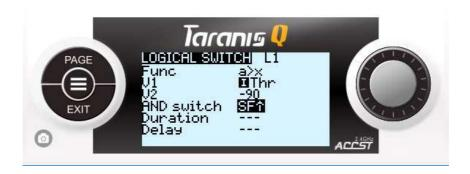
Interpretation: logical switch L1 would be activated if: Thr input is more than -90 and if SF switch (ARM) is at furthest from us (minimum, ON is you set it right in the F3 board) position.
