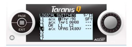
Interpretation: logical switch of line4 would activate when VFAS value would be less than 14.80V
