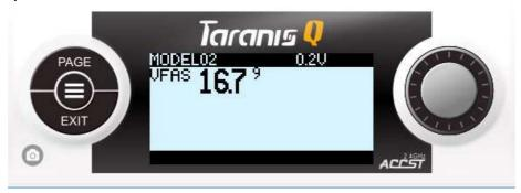
This screen shows you the telemetry values of the sensors that you have added to display on the previous "DISPLAY" page. Add all other telemetry values you want here. Note that each "Nums" screen can display up to 8 values and there could be 4 screens like that assigned to the model. So, 32 sensor values in total for the model. Press "PAGE" to switch between telemetry screens whenever there are more than 1 screen available. Press "EXIT" to back to the main flight screen.
