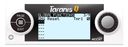
Interpretation: global function of line1 would act as Timer1 reset to the max. desired time set in "SETUP"->"Timer1" model menu when you pull SH momentary switch towards you (max. value).
