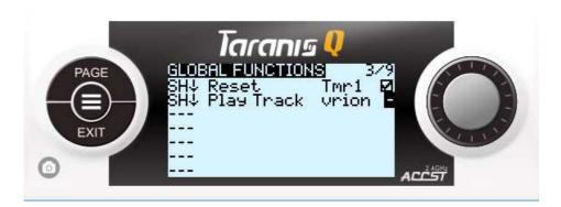
Now, hit "EXIT" until you would get to main flight screen and check how Timer1 and Timer2 perform. Timer1 would start to run when you ARM with SF switch and move Thr stick up to more than -90. It would run until you would pull SH (momentary) switch that would reset Timer1 to 06:00 (or whatever time you have set) and play audio file "reset" or whatever file you have set for this function.
