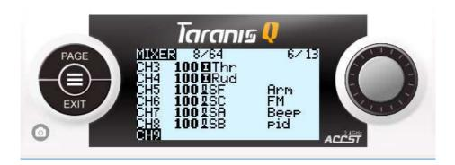
Interpretation: CH8 of the receiver would receive 100% (full range) of SB switch input (-100 (negative endpoint) signal at SB switch at upper position, 0 (center) signal at SB center position and +100 (positive endpoint) signal at SB switch at down position).
