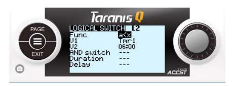
Interpretation: logical switch L2 would be activated if: Tmr1 current countdown time is less than the max. desired time of of the timer1. So, this Logical Switch would work all the way from 05:59 and down to -xx:xx time unless we would reset our timer1 to 06:00.
