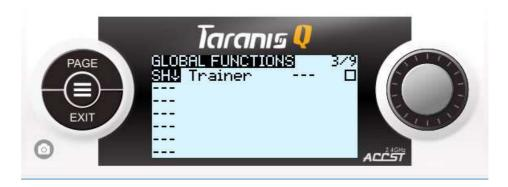
Select next field to the right and set the value to "RESET" and third field value to Tmr1. And put a checkbox in the next field. Press "EXIT" to return exit the line edit.
