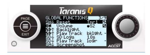
Highlight the first empty line, press "ENTER" and move SH switch towards you to get "SH  $\downarrow$ " reading, press "ENTER" again to save this value.
