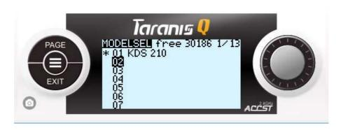
\*note: if you would create a new model – it would automatically have 1<sup>st</sup> 4 channels in the order as you have stated in "RADIO SETUP" menu (in my case AETR). That is why we needed to set this channel order in "RADIO SETUP" according to our preference. The default model that you have on the radio from the factory has another 1<sup>st</sup> 4 channels order. I prefer to delete such models and create a new one.
