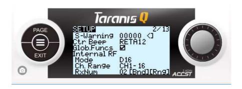
Press and hold BIND button on your receiver, power it up. Release BIND button. Power off the receiver. Press "EXIT" on the radio to leave the BIND mode. Power on your receiver again. This time the green led on the receiver should be constantly lit indicating that there is a connection to the radio.
