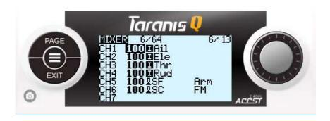
Interpretation: CH6 of the receiver would receive 100% (full range) of SC switch input (-100 (negative endpoint) signal at SC switch at upper position, 0 (center) signal at SC center position and +100 (positive endpoint) signal at SC switch at down position).
