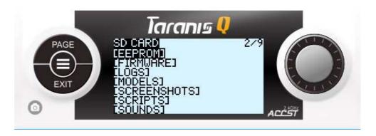
with the right rotary dial navigate to "FIRMWARE" folder, press enter, navigate to the FW file you have here, long press "ENTER" (center rotary dial press) and select Update bootloader. Now, you have your bootloader up to date and with the version corresponding to the radio FW file. Hit "EXIT" several times to get back to the main flight screen.
