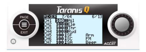
Interpretation: CH7 of the receiver would receive 100% (full range) of SA switch input (-100 (negative endpoint) signal at SA switch at upper position, 0 (center) signal at SA center position and +100 (positive endpoint) signal at SA switch at down position).
