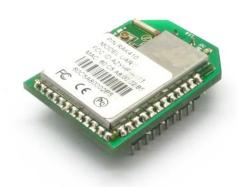
WIFI Bee is a serial port WIFI module that fully supports IEEE 802.11b/g/n wireless standards. It is internally integrated TCP/IP protocol stack and compatible with any Bee socket. It can directly plug into the Bee sockets and use the UART port for communication.
