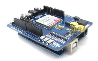
IComsat is a GSM/GPRS shield for Arduino and based on the SIM900 Quad-band GSM/GPRS module. It is controlled via AT commands (GSM 07.07,07.05 and SIMCOM enhanced AT Commands), and fully compatible with Arduino / Iteaduino and Mega.
