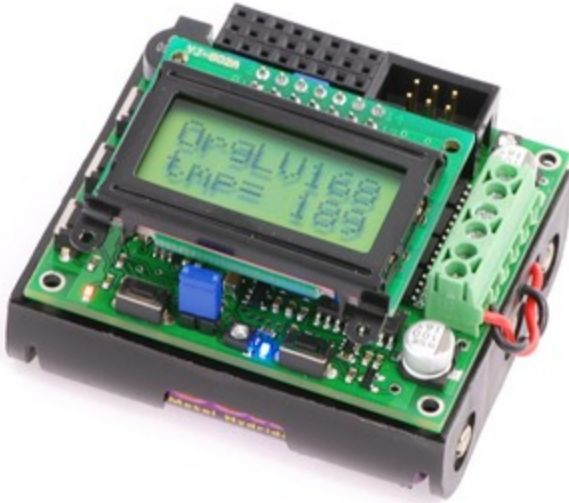
The Orangutan LV-168 attached to a 3-AA battery holder.
