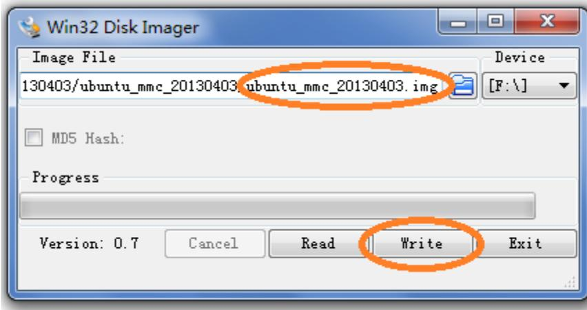
After a few minutes, when the progress bar reach 100%, the TF card is ready to use to bootup the pcDuino.
