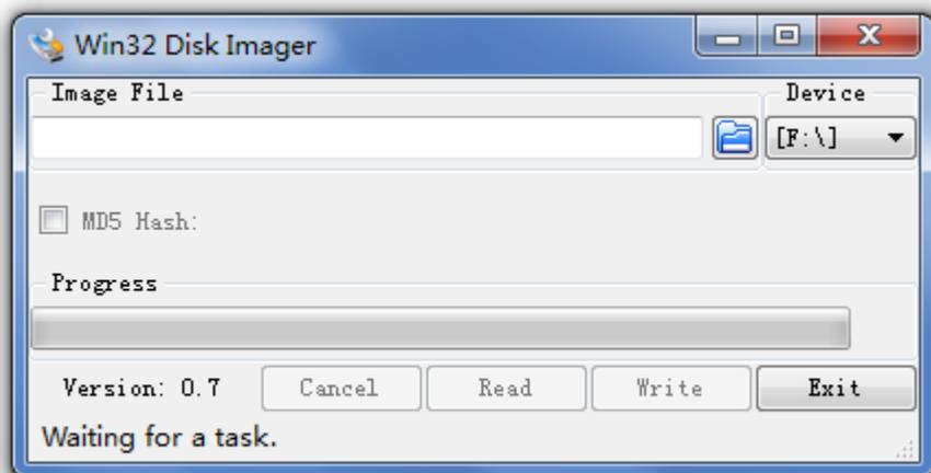
(b) Choose the SD bootable Ubuntu image file ubuntu\_mmc\_xxx.img that you've downloaded and write it to micro-SD card
