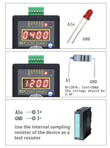
7.2 Connect an LED indicator, if the brightness changes with the adjustment,
