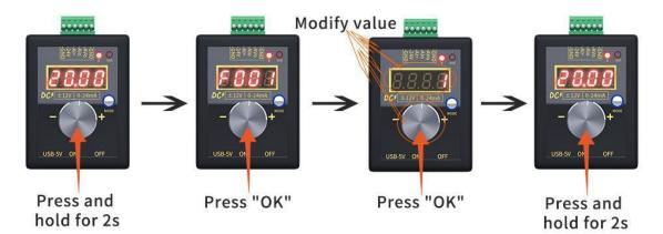
Figure 1 $\rightarrow$ 2: Press and hold the knob for 2 seconds, Enter setting state, Display "F001";
