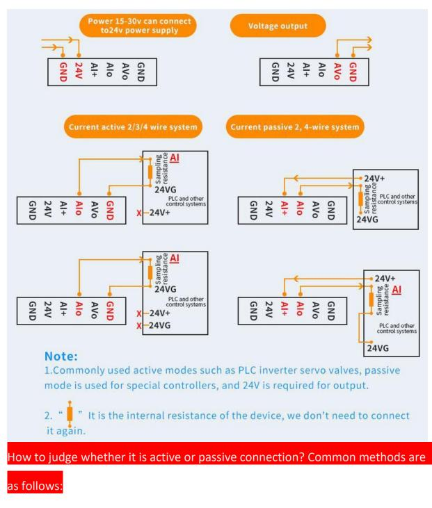
1 : See the internal schematic document of the device, I+ is 24V+, it is the
