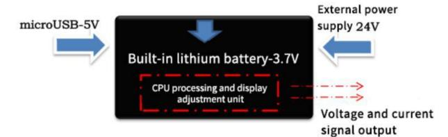
3 power supply methods, as long as one is used, it can work, and it can be connected at the same time;
