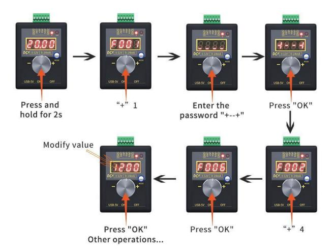
Figure  $1 \rightarrow 2$ : Press and hold the knob for 2 seconds, Enter setting state,
