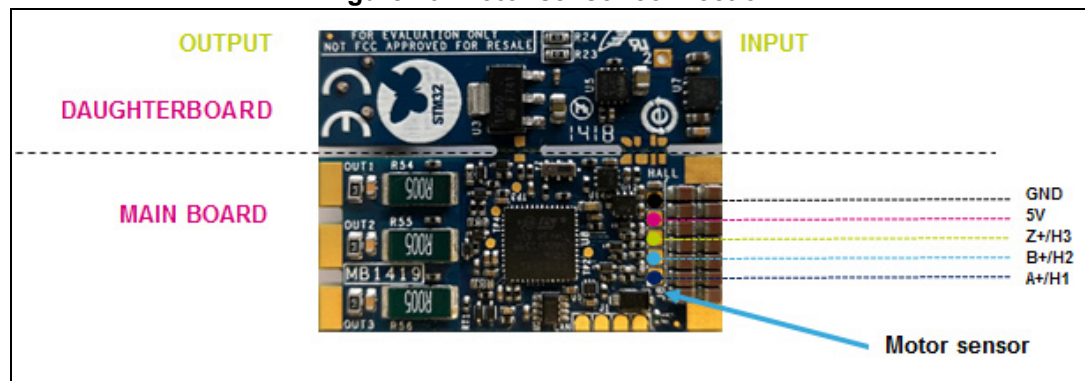
Figure 10. Motor sensor connection
