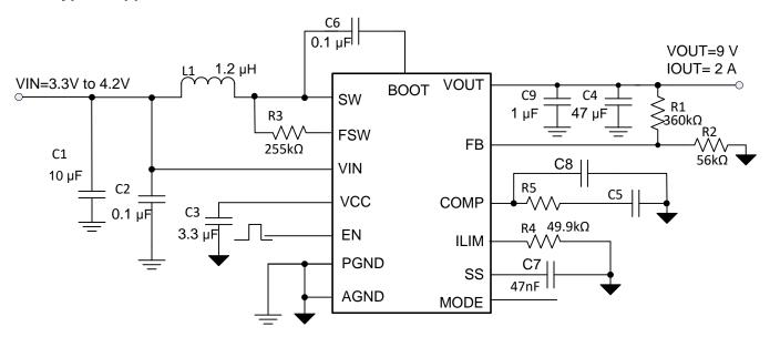
Figure 13. TPS61088-Q1 3.3 V to 9-V/3-A Output Converter
