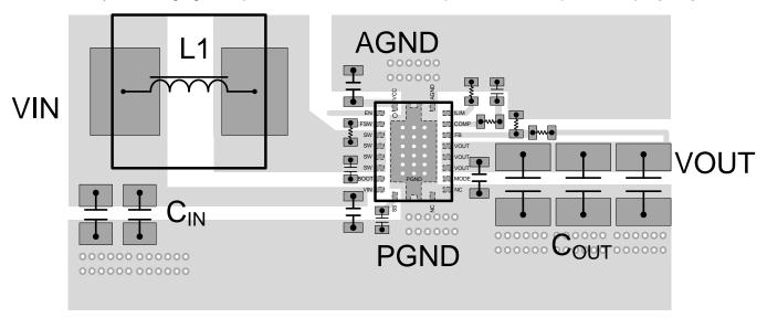
Figure 21. Recommended TPS61088-Q1 Layout
